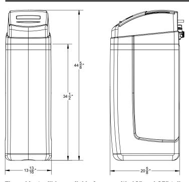
The Water Specialist – CWS-35 Cabinet accepts 35" tall mineral tanks up to a 12" diameter to maximize system capability.
